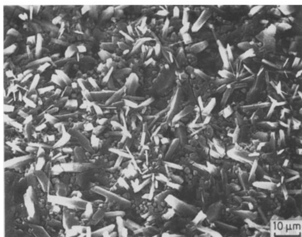
Figure 5 Surface view – cordierite + Na 2 SO 4 :O 2 , 24 h.
