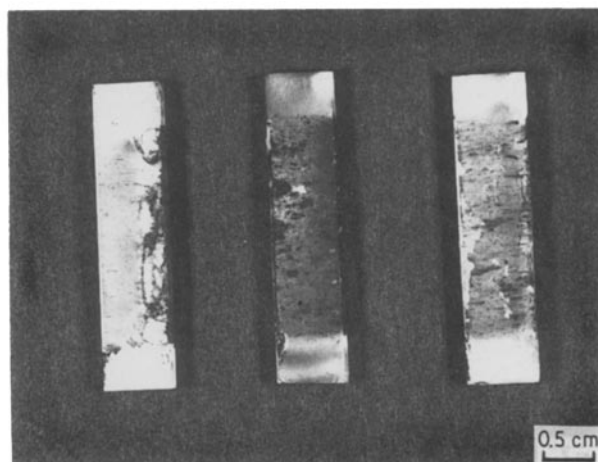
Figure 11 Cordierite corroded in a 4 atm burner rig for 40 h at 1000^\circ\text{C} .
